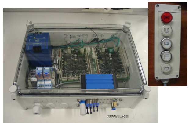
Milkroom Controller Non De Laval tank
