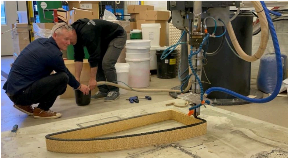
3D printing the modules using biodegradable materials.
